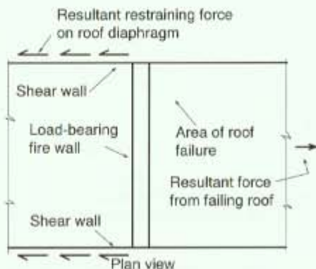
Fig. 2b. Plan view of forces acting during failure.
