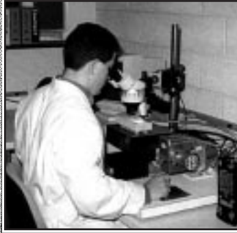
A CTL petrographer utilizes a computerized linear traverse/modified point count system to electronically record and measure air content and other air-void system parameters.
