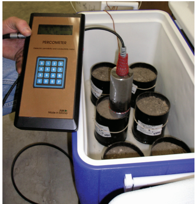
Figure 2.3. The Tube Suction Test measures the movement of water in cement-stabilized materials.
