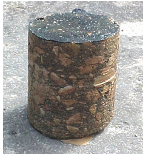
Figure 1.3. Pavement core proves strength of CTB. Even in severe climates the strength of CTB increases due to continued cement hydration.
