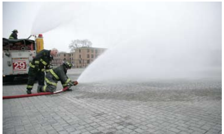
The Chicago Fire Department demonstrates the high surface infiltration rate of permeable interlocking concrete pavement at the U.S. Cellular Field.
