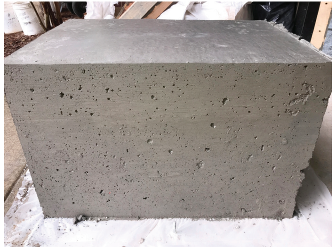
FIGURE 7-4. Laboratory test block of two lifts of IVRCC.
