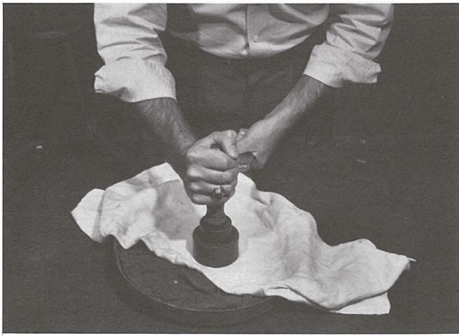
Fig. 16. Giving soil-cement-water preliminary compaction to facilitate moisture distribution in heavy-textured soil.
