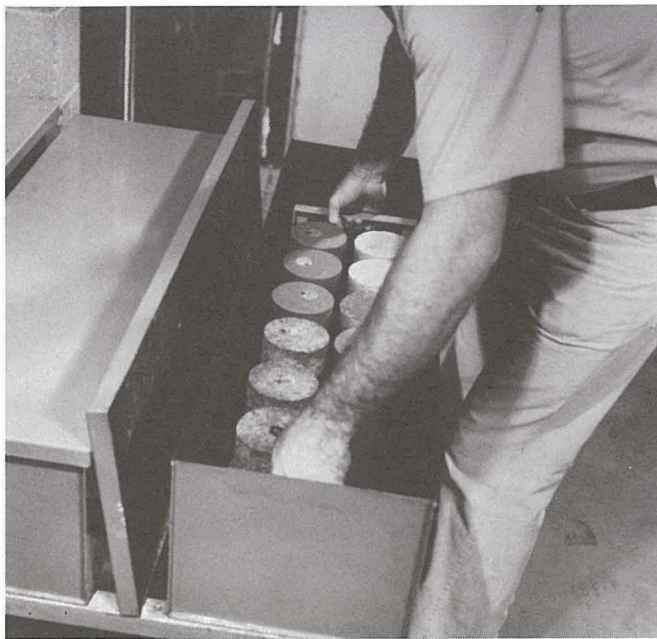
Fig. 28. Freeze-thaw test specimens complete thawing portion of cycle in contact with saturated absorbent pads which supply excess quantities of water that specimens absorb by capillary action.
