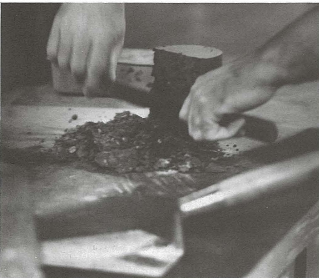
Fig. 12. Taking moisture sample from center plane of specimen during moisture-density test.
