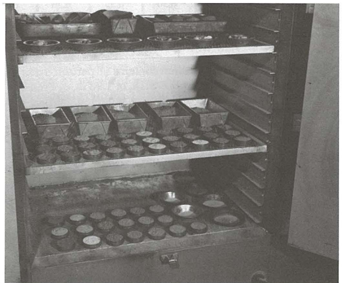
Fig. 13. Moisture samples are dried to constant weight in a thermostatically controlled oven at 110 deg C.
