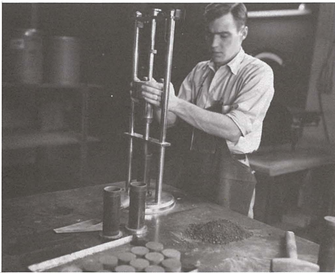
Fig. 30. Molding 2-in. compressive-strength test specimens.
