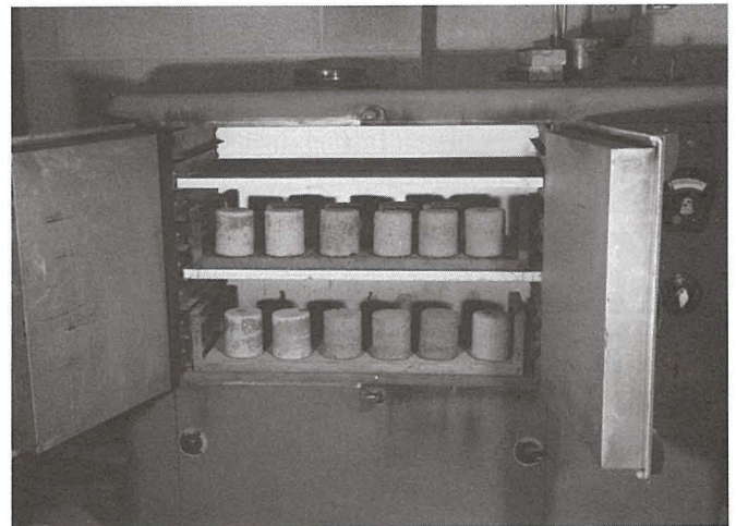
Fig. 24. Forty-two hours' drying at 160 deg F completes cycle of wet-dry test.
