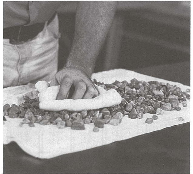
Fig. 9. Surface drying material retained on a No. 4 sieve with towel
