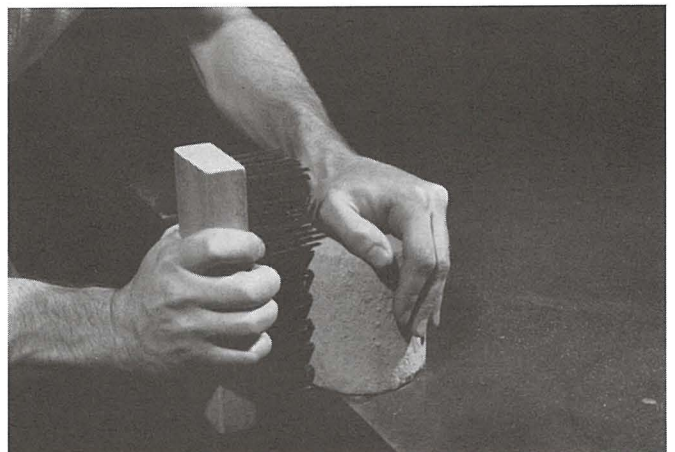
Fig. 25. Soil-cement specimens are given two firm strokes on all areas with a wire scratch brush after each cycle of wetting and drying or freezing and thawing. See Appendix, for specifications for this brush.
