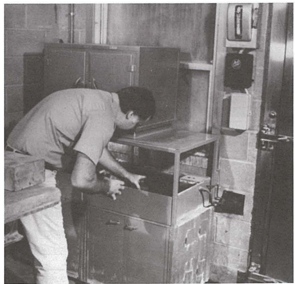
Fig. 23. Wet-dry test specimens are immersed in water for 5 hours each cycle.
