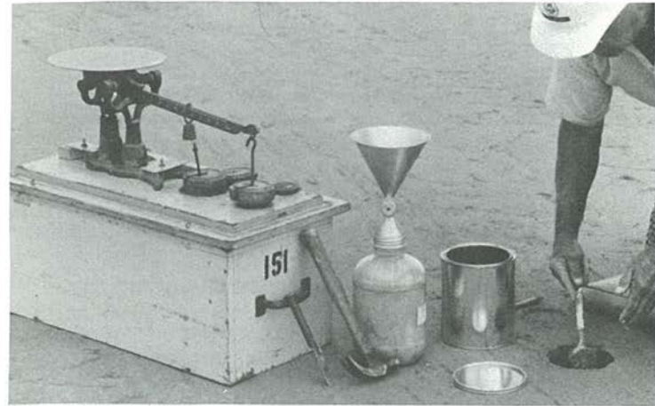
Fig. 26. Density of compacted soil-cement being determined by the sand-cone method. A hole is dug in the base, and the dry weight of the material removed and the volume of the hole are computed.
