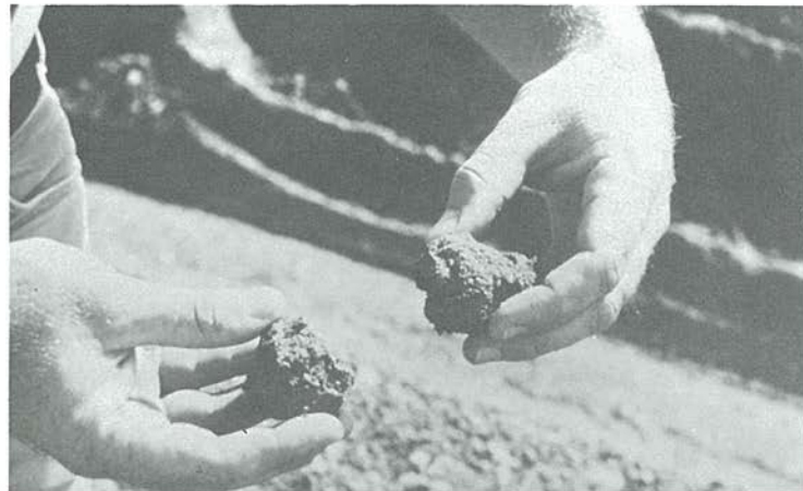
Fig. 21. Soil-cement at optimum moisture casts readily when squeezed in the hand and can be broken into two pieces without crumbling.
