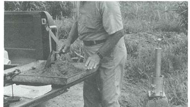
Fig. 15. Running a field moisture-density test.
