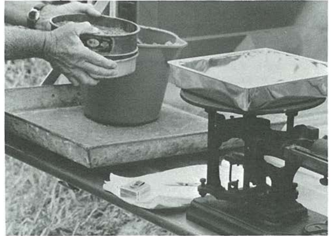
Fig. 4. Screening soil-cement mixture through No. 4 (4.75-mm) sieve to determine percent pulverization.
