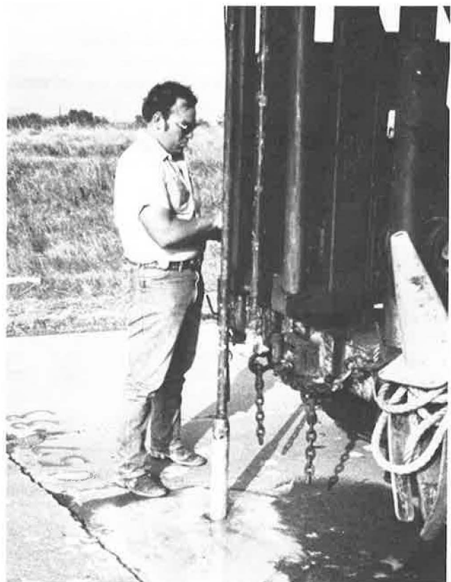
FIGURE 2 Thin-walled tube sampling the soil.
