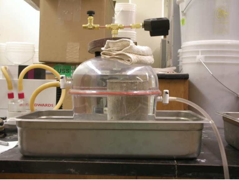
Figure 8. Vacuum saturation test configuration.
