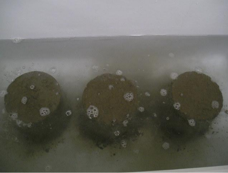
Figure 7. Soaking configuration for freeze-thaw testing.
