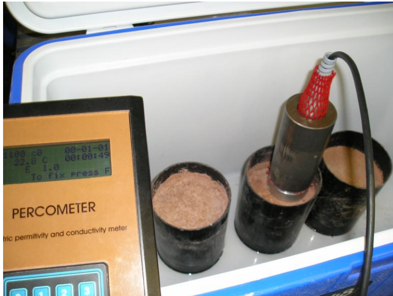
Figure 10. Tube suction test configuration.
