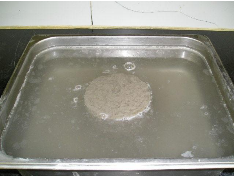
Figure 4. Specimen soaking prior to UCS testing.
