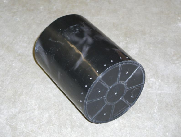
Figure 9. Plastic mold used for tube suction test.
