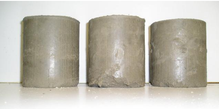
Figure B22. Clay specimens treated with 1 percent cement after 0 cycles of freeze-thaw testing.
