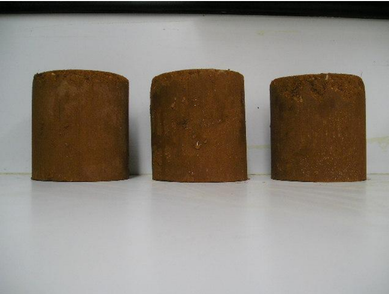
Figure 6. Thawing configuration for freeze-thaw testing.
