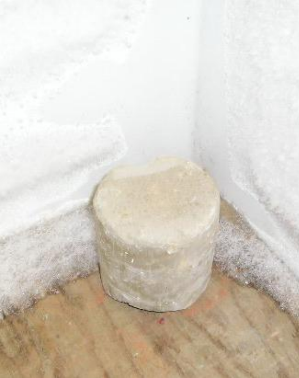
Figure 5. Freezing configuration for freeze-thaw testing.
