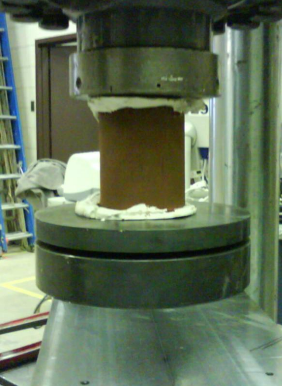
Figure 2. UCS test machine.
