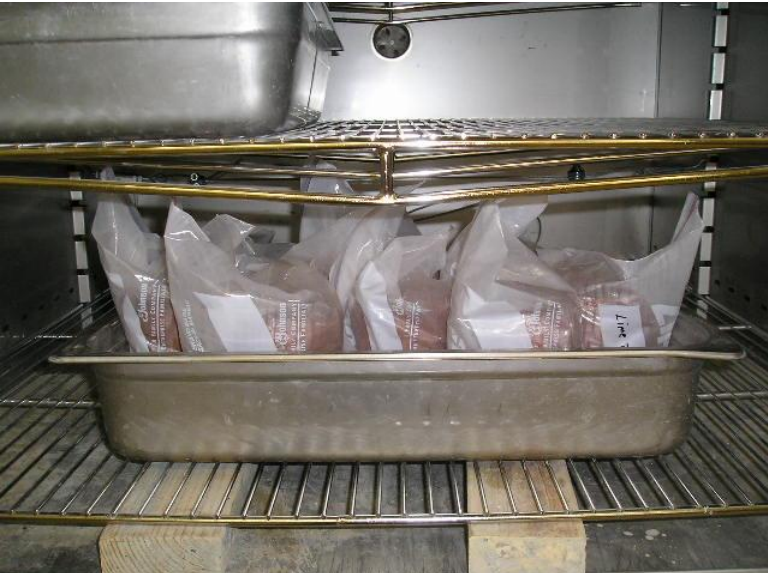
Figure 3. Curing conditions for specimens treated with fly ash and/or lime.
