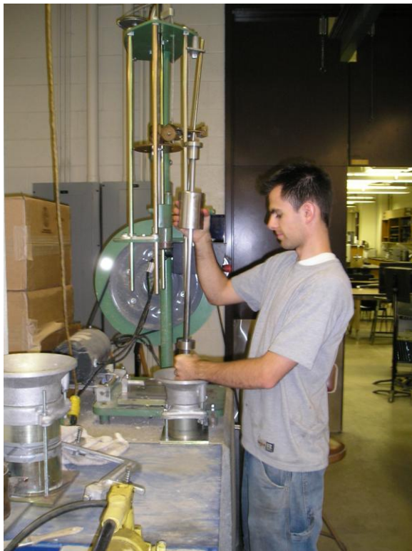
Figure 1. Compaction apparatus and finishing tool.
