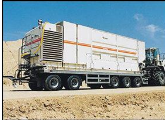
Figure 1.8. Wirtgen Mobile Slurry Mixing Plant. Note: photo courtesy of the Wirtgen Group.
