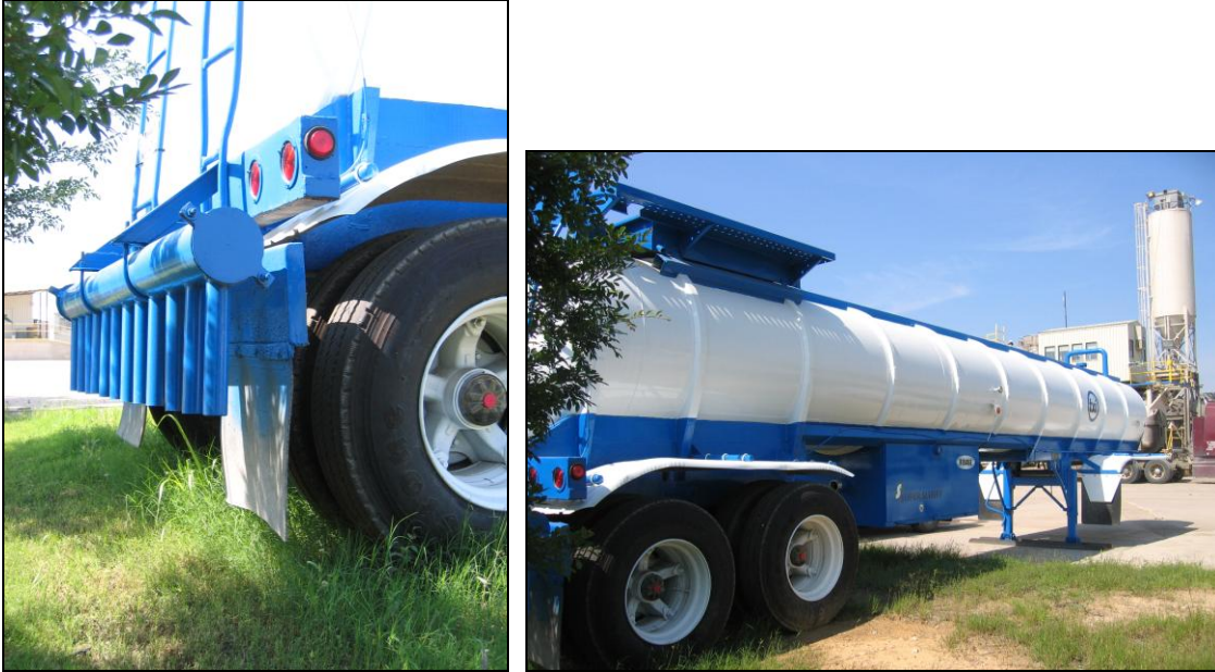
Figure 1.2. Haul Trailer for Transporting and Spreading Super Slurry.
