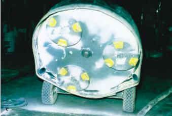
Figure 20. (a) Polished terrazzo floor. (b) Rustic terrazzo (c) Diamond embedded abrasive pads of varying fineness (d) Hand-held planetary grinder (e) Buffer-size planetary grinder. (l to r, 70873, IMG7075, NA, NA, NA)
