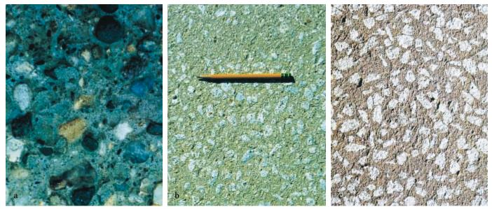
Figure 19. Exposed-aggregate surfaces produced by (a) sandblasting, (b) scarifying, and (c) bushhammering. (IMG: 7071, 7072, 7073)
