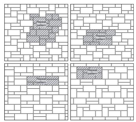
Figure 53. Illustration of various ashlar patterns that can be produced using the technique shown in Figure 52.
