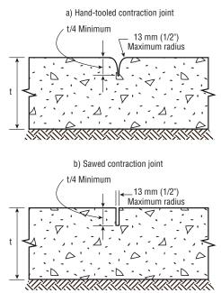
Figure 72. If the groove is to serve as a contraction joint, a groover with a bit deep enough to cut the slab a minimum of one-fourth its depth is mandatory. A shallow groover may be used for decorative scoring.
