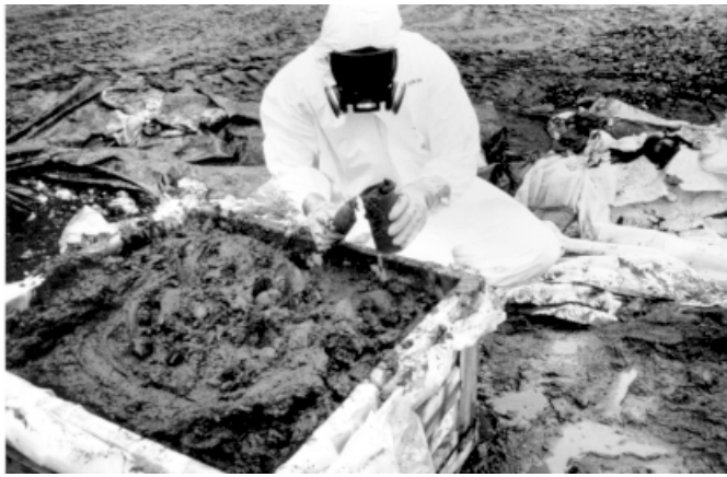
Fig. 15. Sampling S/S mixture for testing. (Courtesy EPA)
