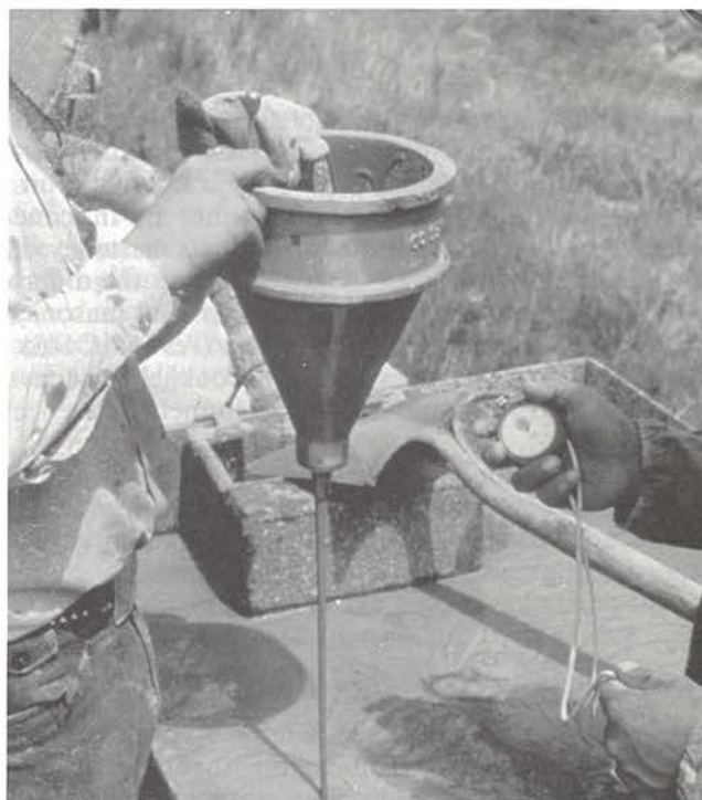
Fig. 1. (a) Cross section of flow cone for measuring consistency meeting ASTM C 939 and Corps of Engineers CRD-C611. (b) Grout discharge and timing to determine efflux time or time of flow (time it takes the grout to discharge from the cone).
