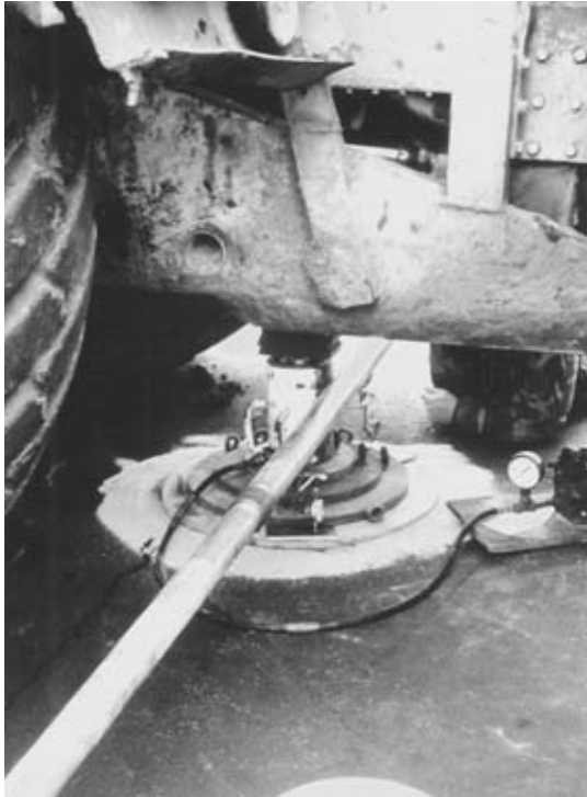
Figure 12. Plate load testing with a standard 30 in. (760 mm) diameter plate.
