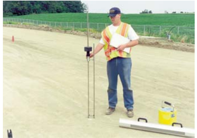
Figure 13. Cone penetrometer testing (Minnesota Department of Transportation).
