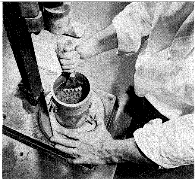
Fig. 8. Scarifying top of first and second compacted layers to remove smooth compaction planes.
