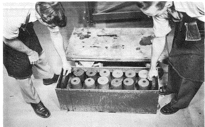
Fig. 14. Wet-dry test specimens are immersed in water for 5 hours of each cycle.
