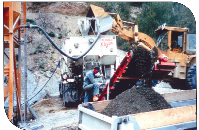
Figure 6—Mobile Truck Mixer.
