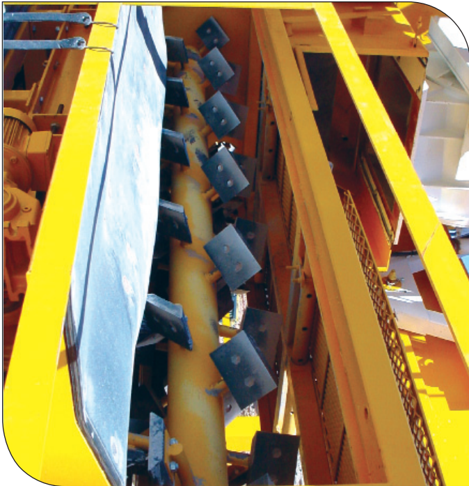
Figure 8—View of Pugmill Mixing Chamber.
