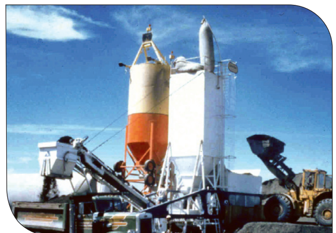
Figure 7—Continuous Flow Pugmill Mixer.
