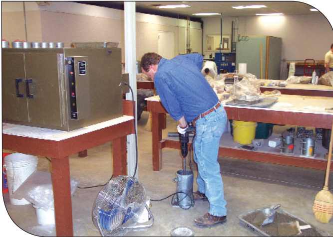
Figure 3—Preparing RCC Samples According to ASTM C 1435.
