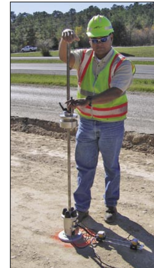
A portable FWD (PFWD) provides a compact alternative to the standard FWD for controlling microcracking. Other stiffness devices may also be able to control microcracking.
