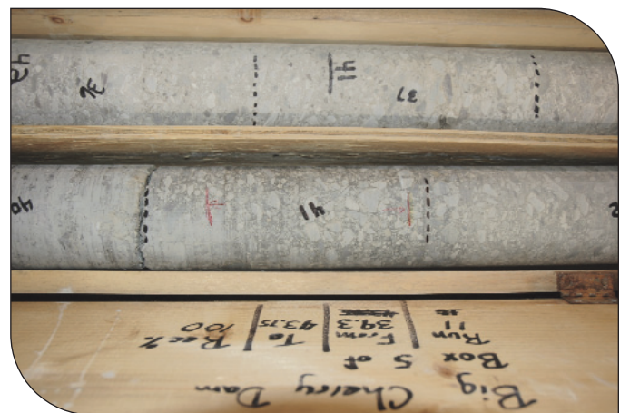
RCC core extracted from the new dam
