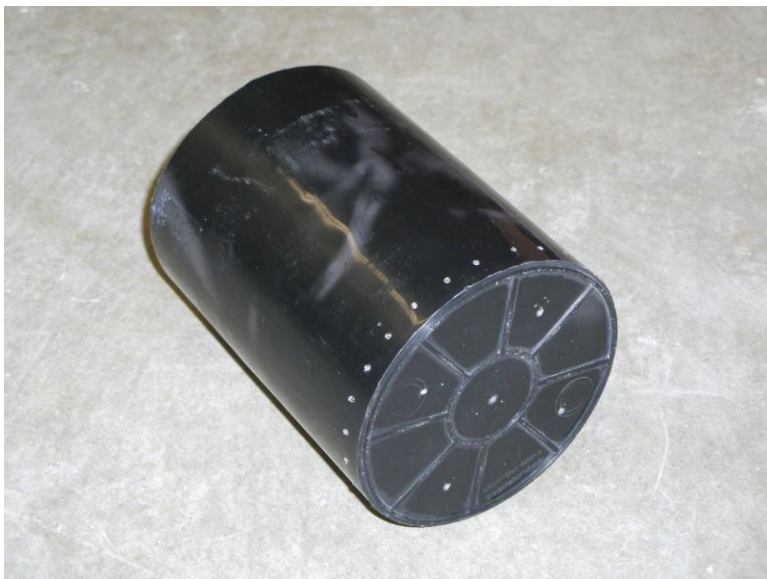
Figure 12. Plastic mold used for tube suction test.
