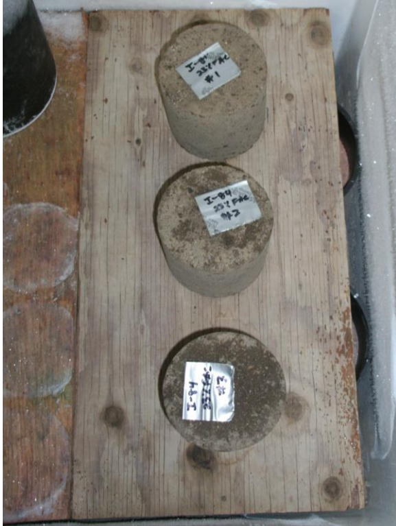
Figure 7. Freezing configuration for freeze-thaw testing.
