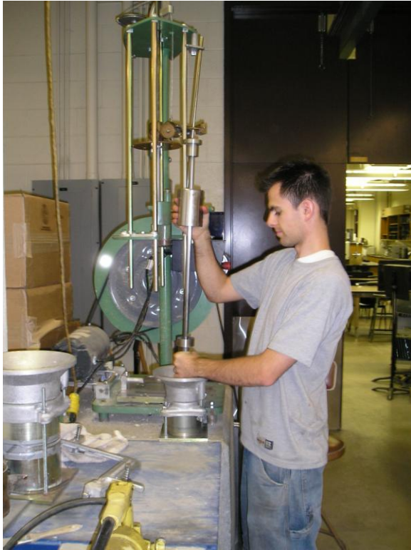
Figure 1. Compaction apparatus and finishing tool.
