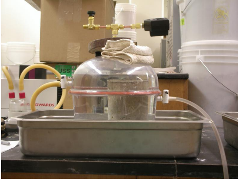
Figure 11. Vacuum saturation test configuration.
