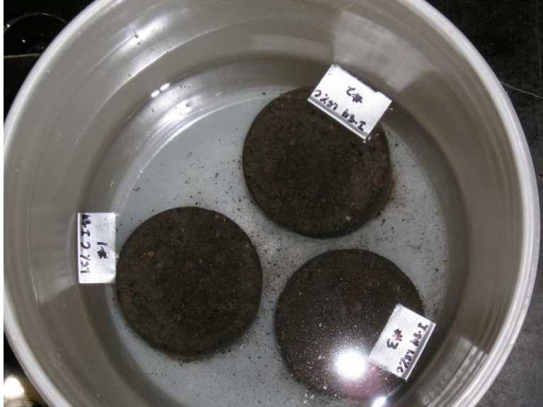
Figure 6. Specimens soaking prior to UCS testing.
