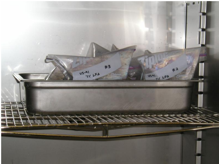
Figure 5. Curing conditions for specimens treated with Class C fly ash and lime-fly ash.
