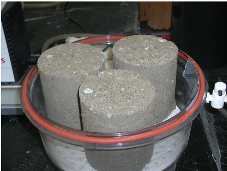
Figure 10. Vacuum chamber used for vacuum saturation test.
