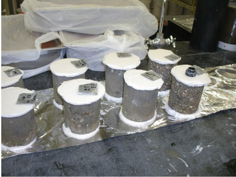
Figure 3. Specimens capped for UCS testing.
