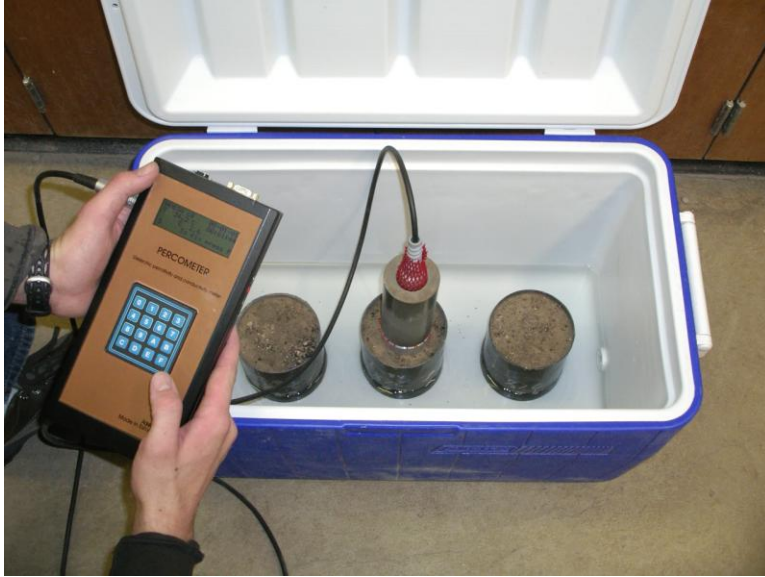
Figure 13. Tube suction test configuration.
