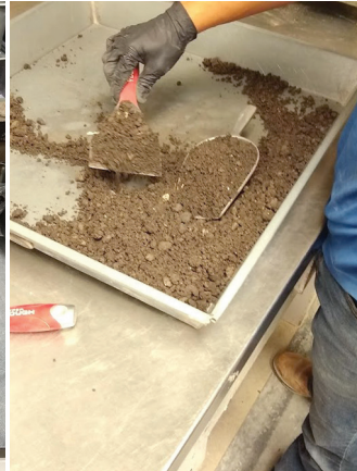
Figure B.2. Mixing additive and soil in the laboratory
