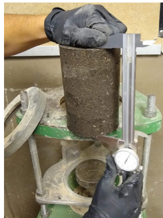
Figure B.7. Measuring the height of a specimen using a micrometer dial assembly
