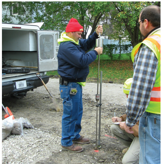
Figure 3.7. Dynamic cone penetrometer testing
