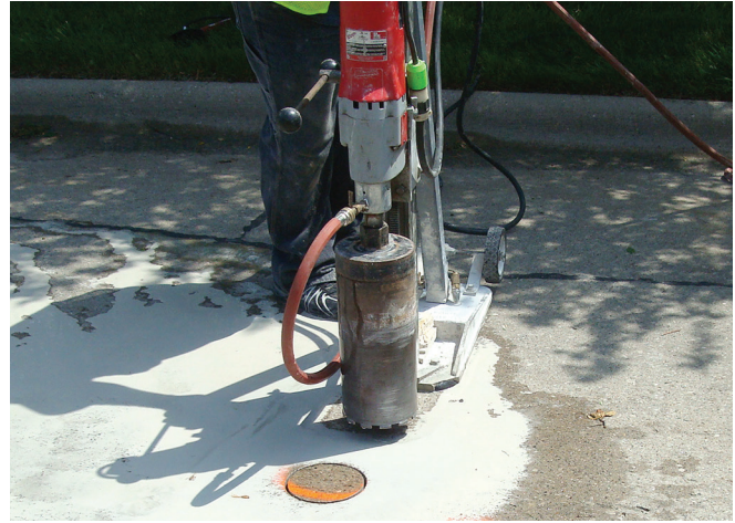
Figure 3.3. Core sampling of pavement
