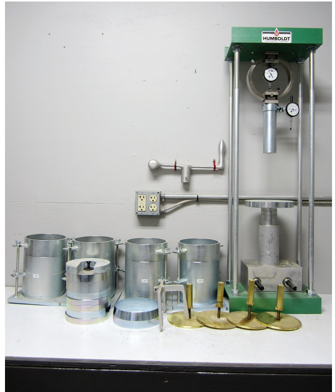
Figure 2.6. CBR testing machine
