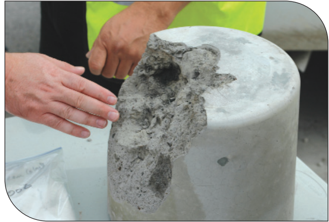
Cleaved “bucket cast” of treated soil. Note coal tar inclusions.
